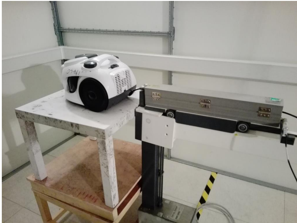
Photograph 3: Set-up for Disturbance Power on AC mains
