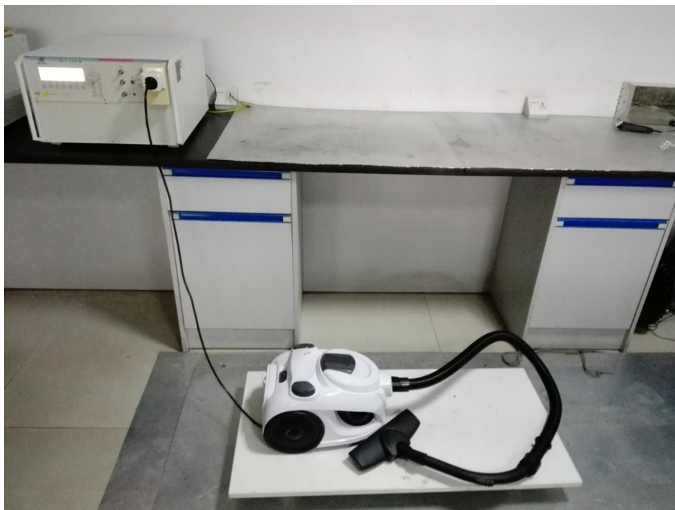
Photograph 7: Set-up for Surge and Voltage Dips and Short Interruptions
